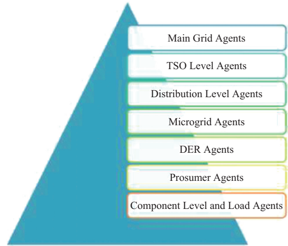
Fig. 6. Seven layered agent-based control structure of smart grid (TSO: transmission system operator).
